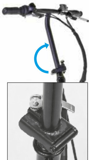
Fold up the Stem and lock in place with the quick-release clamp
