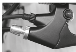
Applying the brakes activates the brake sensor which cuts the power to the motor.
